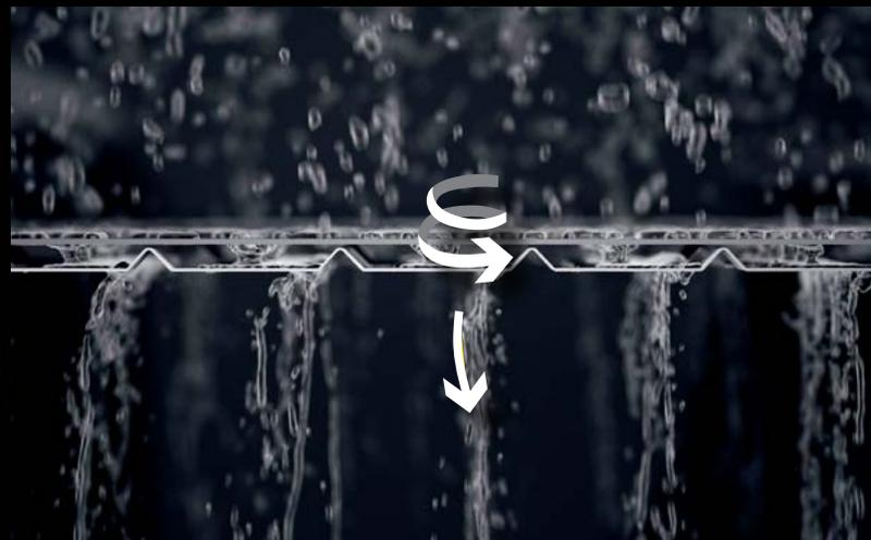
With the **vortex<sup>™</sup>** TECHNOLOGY, the suction created by the two membranes makes it possible to drain three times more water than recorded in the heaviest storms.
